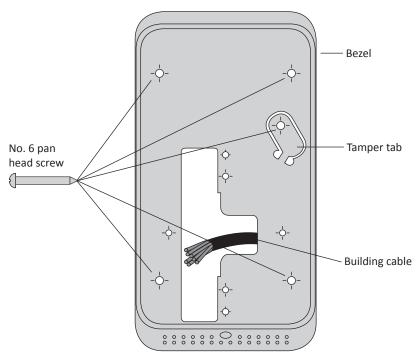
6. Connect the terminal tail extending from the facia assembly to the building cable. Connect the wires for the appropriate device you wish to interface, either an HBUS device or a Cardax IV device, as shown:
