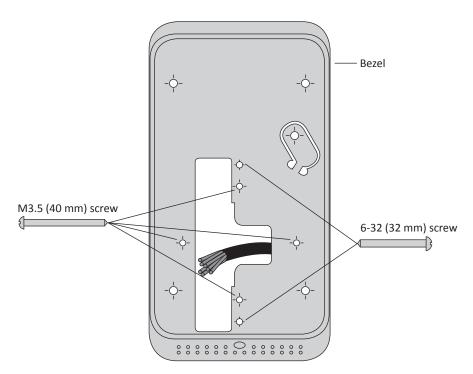
5. Drill pilot holes for the four corner fixing holes and the tamper tab. Secure the bezel to the mounting surface using the four corner fixing screws provided. Secure the tamper tab (located in the bezel) to the mounting surface using the remaining fixing screw provided. It is important the four corner fixing screws are used to ensure the terminal is flush with and tight against the mounting surface.
