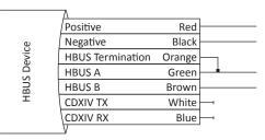
**Note:** To terminate an HBUS terminal, connect the **Orange** (HBUS Termination) wire to the **Green** (HBUS A) wire.
