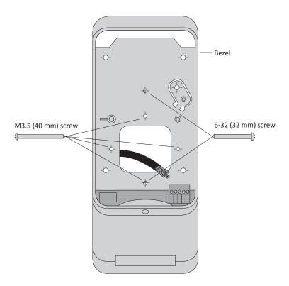
4. Drill pilot holes for the four corner fixing holes and the tamper tab. Secure the bezel to the mounting surface using the four corner fixing screws provided. Secure the tamper tab (located in the bezel) to the mounting surface using the remaining fixing screw provided. It is important the four corner fixing screws are used to ensure the reader is flush with and tight against the mounting surface.
