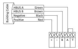
If the reader is the end device on the HBUS cable, terminate the reader by connecting a short piece of wire between terminals T and A.
