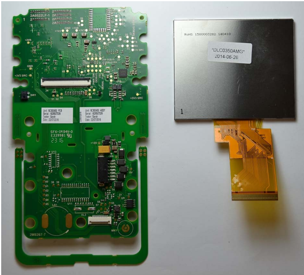
T20 Mifare - PCB (rear side) and LCD
