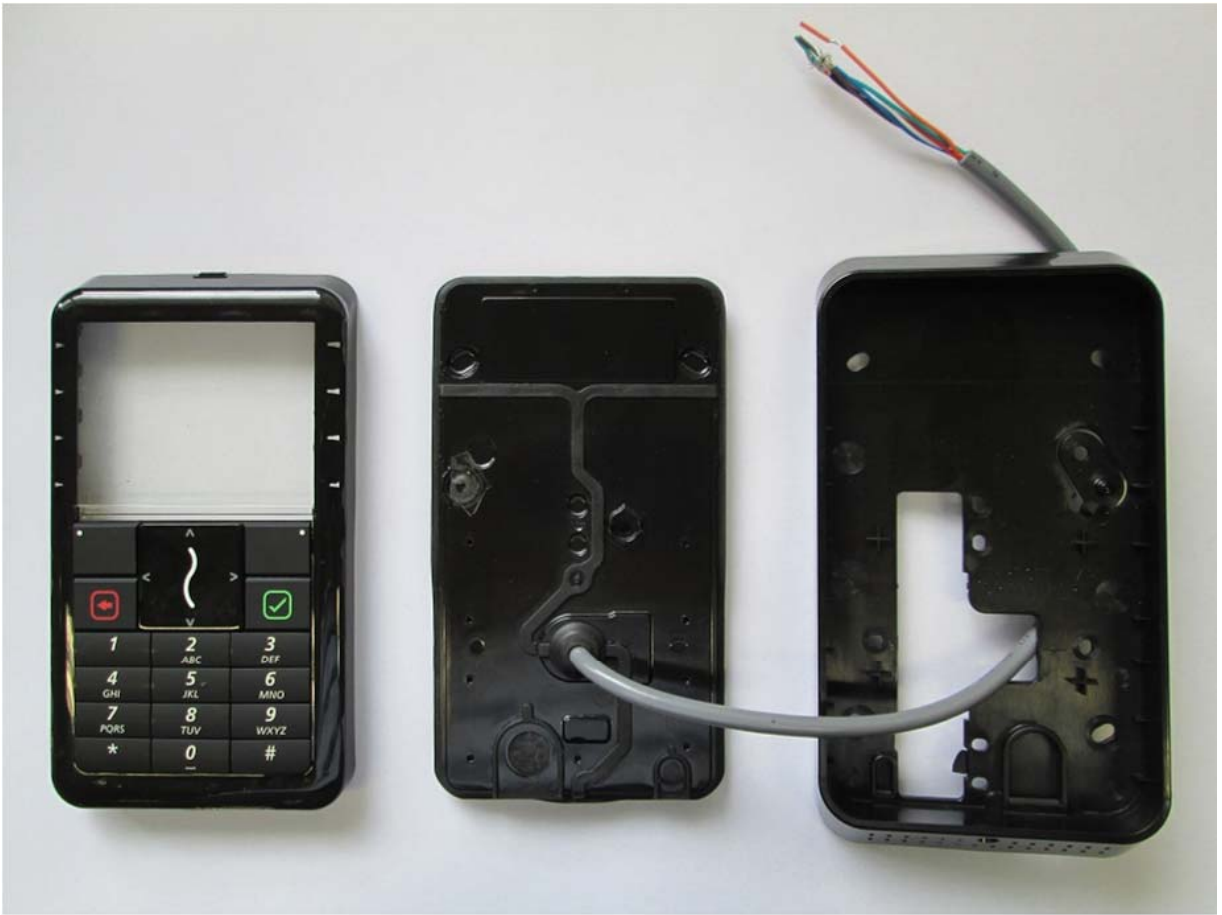
T20 Mifare - Front Case with Keypad, Back Cover with Connection Cable and Mounting Bracket
