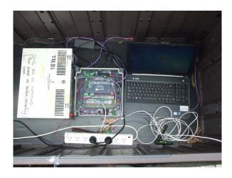
Conducted emissions test set up
