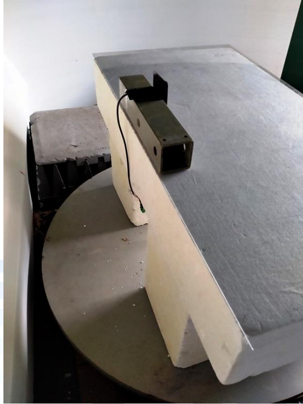
Test Antennas Used – Horn Antenna
