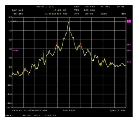
The 99% power bandwidth was then measured using a resolution bandwidth of 10 kHz which is 1% of the occupied bandwidth of 1.106 MHz with measurements being made at the -23 dB points which give a bandwidth of 442.5 kHz
