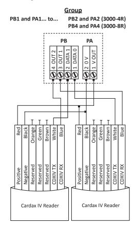
Note: Within each group, you cannot mix Cardax IV Readers with Wiegand Readers. This is because connecting one Wiegand Reader requires all four pins on plug PB. For example, if you connect a Cardax IV Reader to Port 1 of Group 1, Port 2 of Group 1 can only connect to another Cardax IV Reader.
