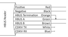
**Note:** To terminate an HBUS Reader, connect the **Orange** (HBUS Termination) wire to the **Green** (HBUS A) wire.
