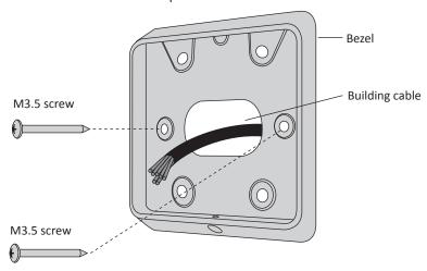
4. Connect the reader tail extending from the facia assembly to the building cable. Connect the wires for the appropriate reader you wish to interface, either an HBUS Reader or a Cardax IV Reader, as shown in the following diagrams.
