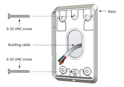
If you are not mounting to a flush box, secure the base to the mounting surface using the four fixing screws provided.
