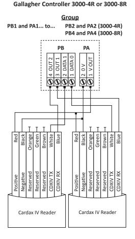
Make the connections from the Gallagher T11 Reader to either the Gallagher Controller 3000-4R or 3000-8R as shown:
