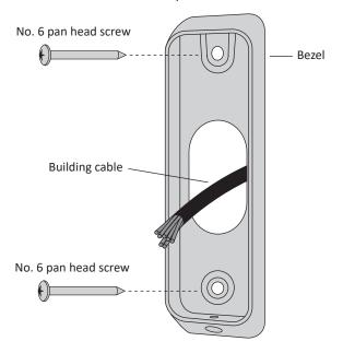
4. Connect the reader tail extending from the facia assembly to the building cable. Connect the wires for the appropriate reader you wish to interface, either an HBUS Reader or a Cardax IV Reader, as shown.
