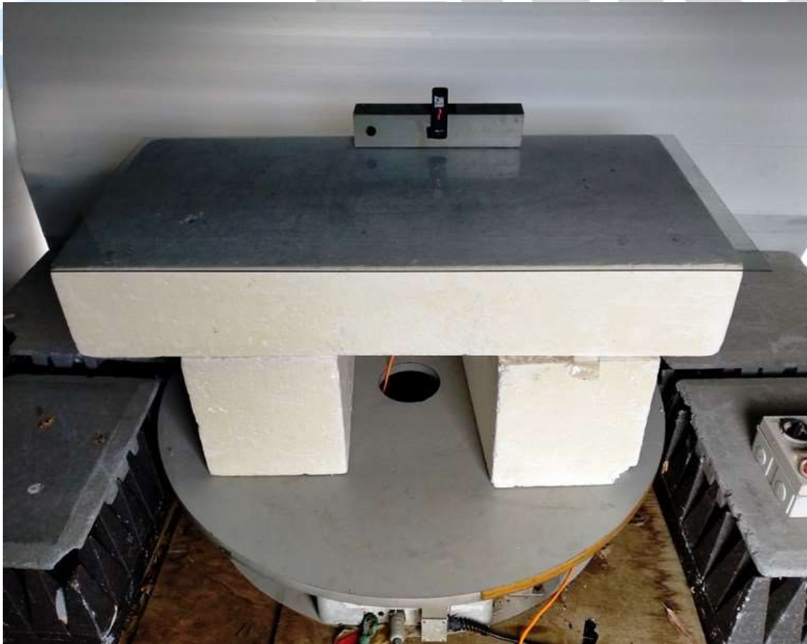
Radiated emission test set up
