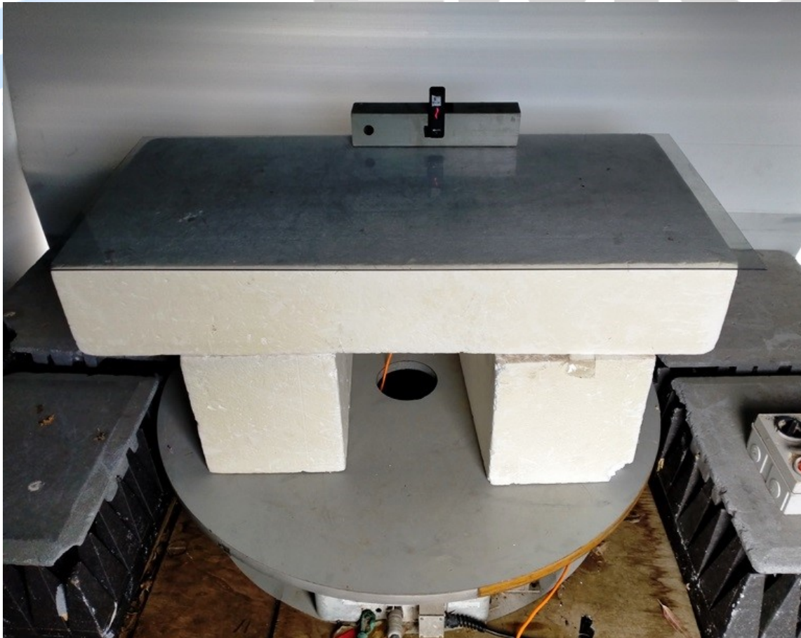
Radiated emission test set up
