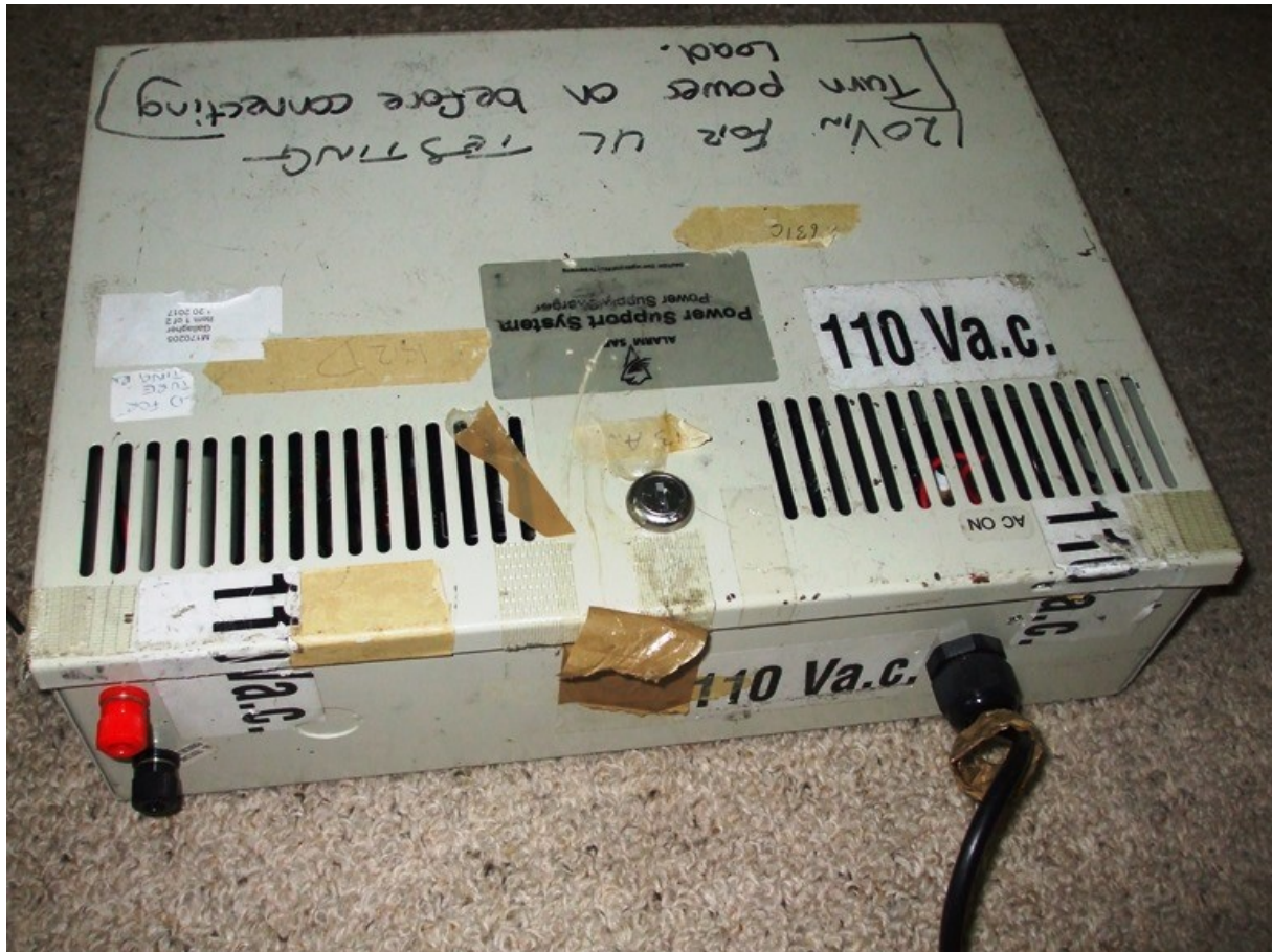
Figure-3: AC to DC convertor (Ancillary)
