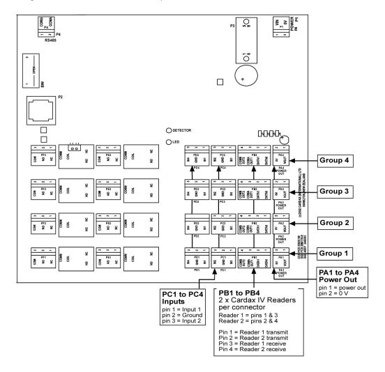
Make the connections from the Gallagher T11 Reader to either the Cardax FT Controller 3000-4R or 3000-8R as shown:
