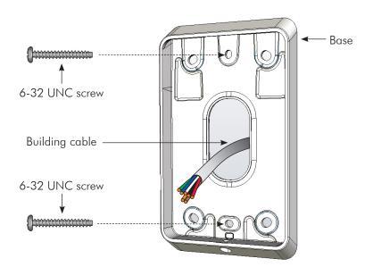
Connect the reader tail extending from the facia assembly to the building cable. 4. Connect the wires shown below.
