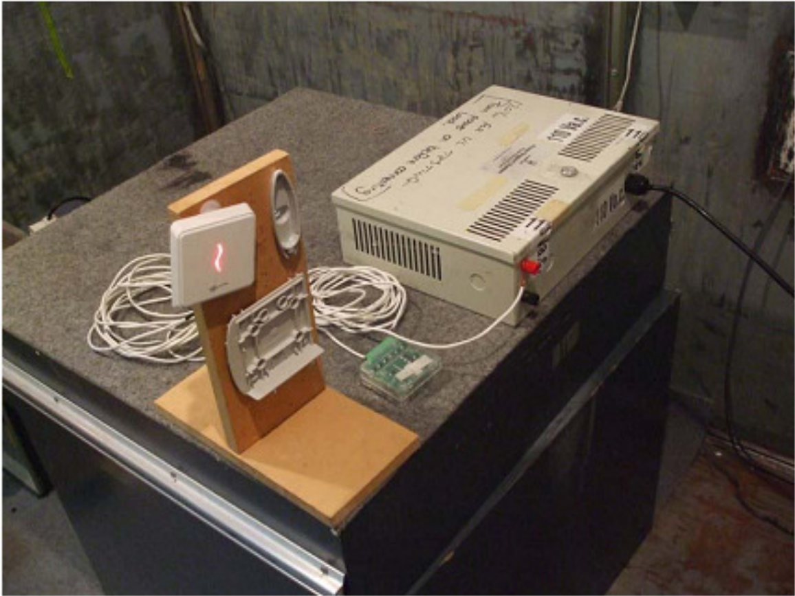
Conducted emissions test set up photos
