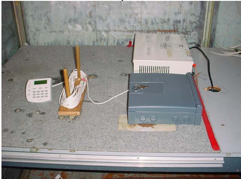
Conducted emissions test set up which includes the ancillaries
