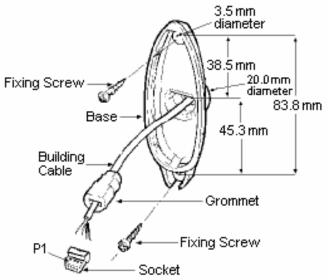
**Note:** The grommet through which the cables feed into the base of the Prox Mifare Series (Teardrop) reader helps to keep the unit waterproof.
