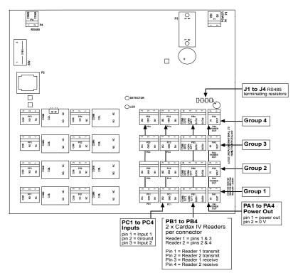
Make the connections from the Prox Mifare Series (Teardrop) reader to the Cardax FT Controller 3000 as shown:
