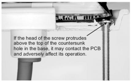
Please note that the manufacturers warranty is voided if the electronics are damaged as a result of the incorrect screws being used or installed incorrectly
