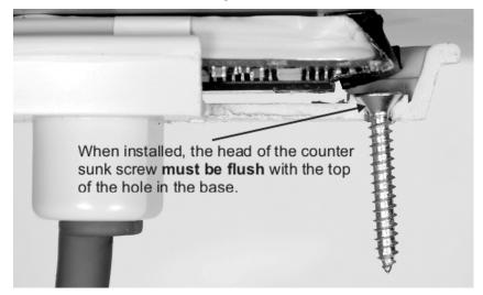
Failure to do this, and/or using other types of screws could interfere with the electronics.
