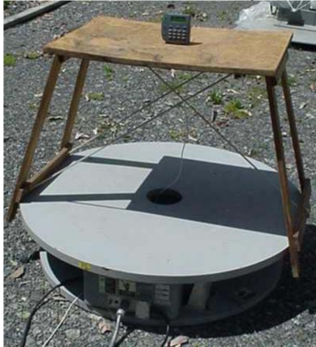
Radiated emissions test set up
