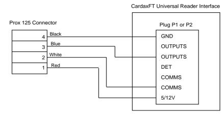
Connect the Prox 125 connector to either the P1 or P2 plug on the CardaxFT URI. Refer to the CardaxFT URI component layout diagram, below, for the location of the plugs.
