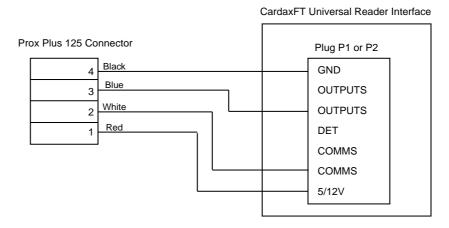
Connect the Prox Plus 125 connector to either the P1 or P2 plug on the CardaxFT URI. Refer to the CardaxFT URI component layout diagram, below, for the location of the plugs.
