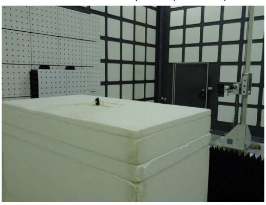
Radiated Emission Set up Photos (Front View)
