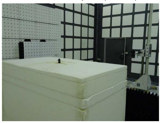
Radiated Emission Set up Photos (Front View)
