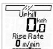
The rate of ascent shows you the vertical, current speed in meters/feet per minute. This means that you can quickly work out how much time you need to get to the summit. This involves a current function, similar to speed.
