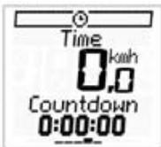
The stopwatch is started and stopped with the top right-hand button. You can use the left button to reset the stopwatch to zero. The stopwatch runs independently from the ride time and must therefore be manually started and stopped.
