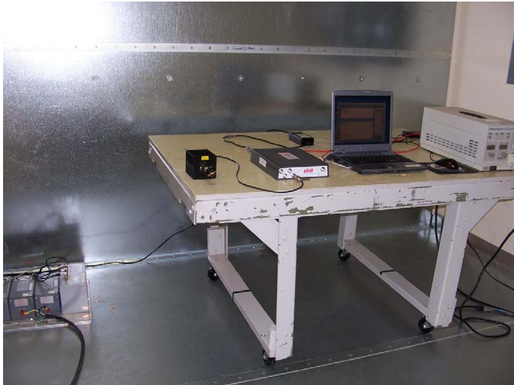
Figure 5 – Test set-up for conducted emissions on AC Mains.
