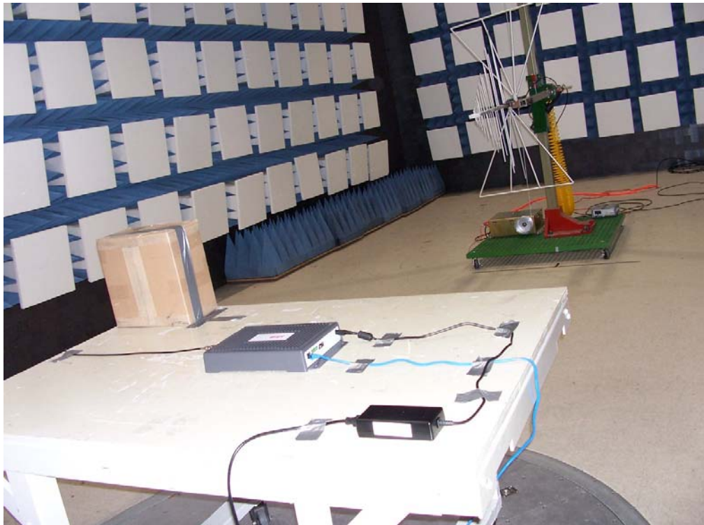
Figure 2 - Radiated Emissions Test Setup
