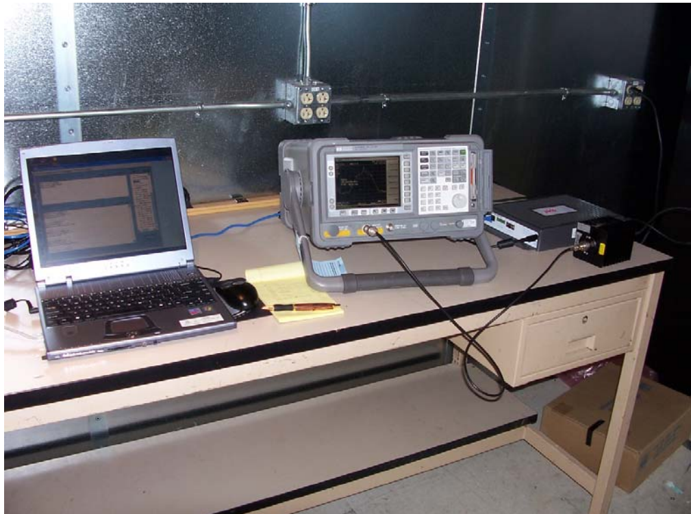
Figure 6 – Typical test set-up for conducted RF Measurements.
