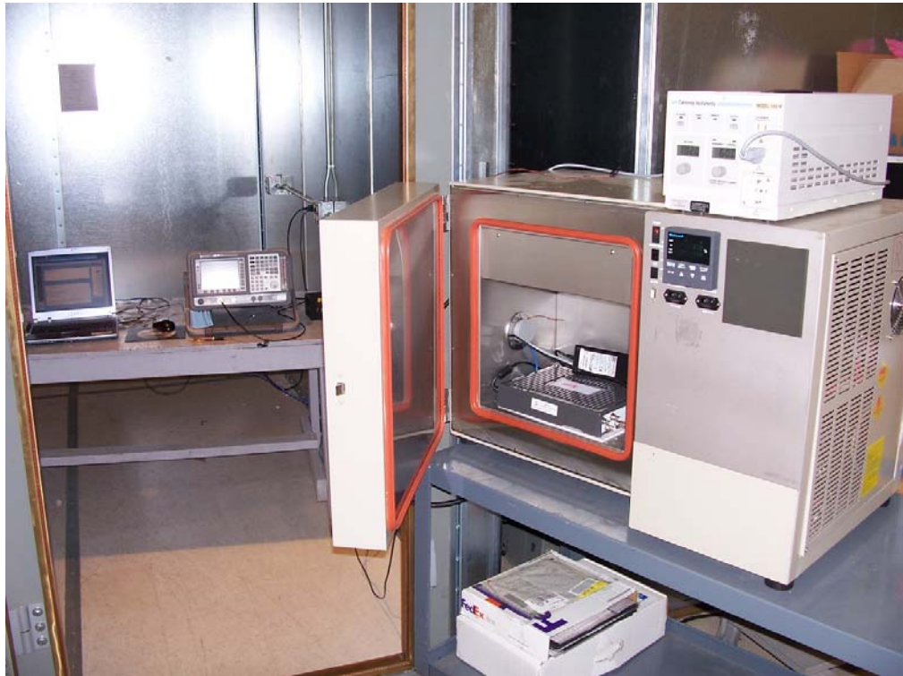
Figure 7 – View of Temperature Chamber Setup and extreme voltage test setups
