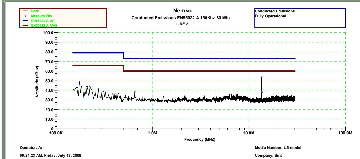
**NOTE:** The peak measured emission levels meet the average limit. The peak emission on the neutral conductor is 60.04 dBuV (peak) at 13.56 MHz.
