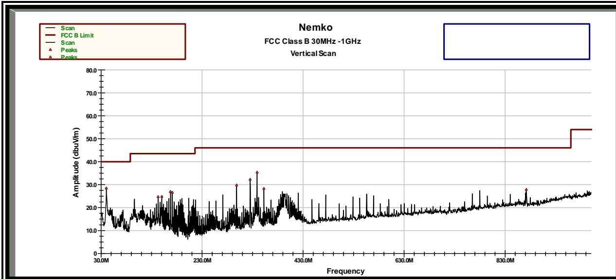
**Test Data - Radiated Emissions****Measurements Above 30 MHz (continued)**
