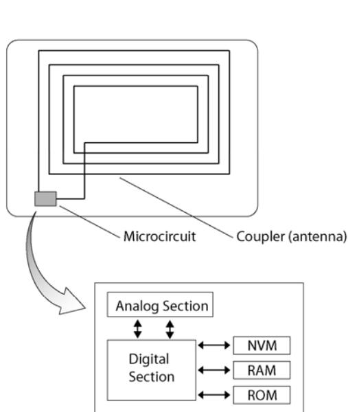
The tag communicates with the reader across the air-interface. This interface is defined by its carrier frequency, bit data rate, encoding method and other parameters.
