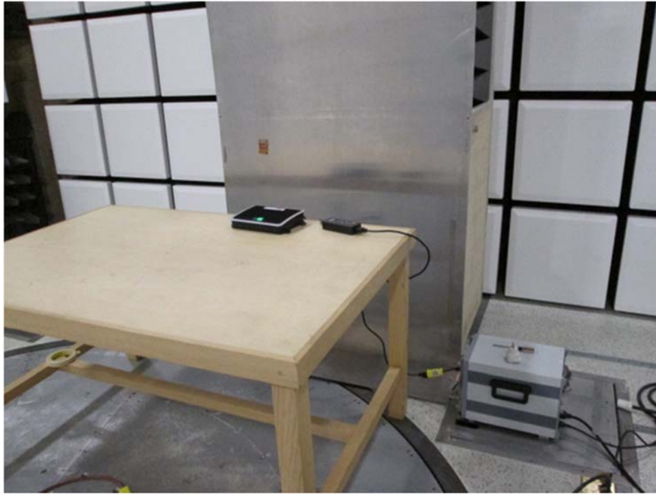
Test Set Up Photo – Line conducted Emissions
