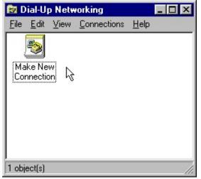
c. In the **Make New Connection** window, input the name of the connection and select Z-Card 210 CDPD Modem (in the type of the modem). Then select **Next** to view the next window.
