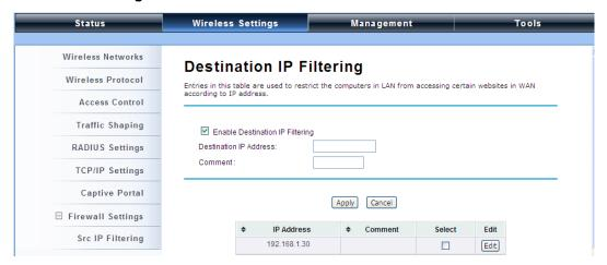
You may create and activate a rule that filters a packet based on the destination IP address to restrict the local computers from accessing certain websites. Check "Enable Destination IP Filtering" to activate rule.
