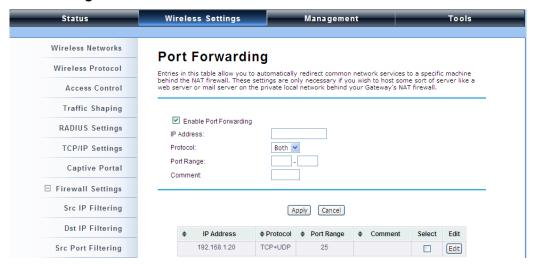
The port forwarding allows you to automatically redirect common network services to a specific machine behind the NAT firewall. These settings ne are only necessary if you wish to host some sort of server like a web server or mail server on the private local network behind IEEE 802.11n Wireless ZAC Wireless CPE's NAT firewall.
