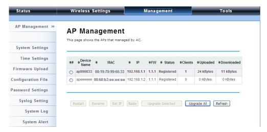
The ZAC Wireless CPE AP in Virtual AC+Thin AP mode on the list is highlighted in bold font. By selecting it and hitting **Radio** button, you may check radio setting such as **channel bandwidth**, **channel**, **antenna** and **output power**.
