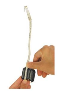
Loop the cable around and through the core. This helps "lock" the core in place, and may be required in circumstances with severe interference.
