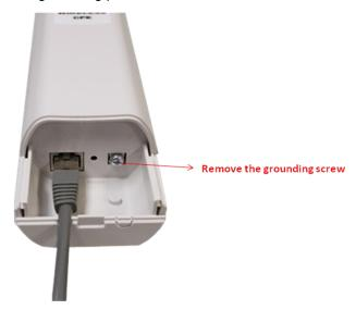
2. Put the grounding wire on the grounding point at the bottom of the ZAC Wireless CPE. Then screw the grounding wire to tighten up.
