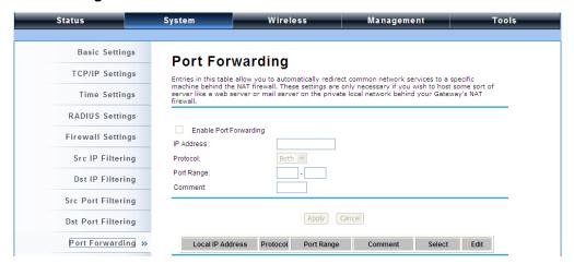
The port forwarding allows you to automatically redirect common network services to a specific machine behind the NAT firewall. These settings ne are only necessary if you wish to host some sort of server like a web server or mail server on the private local network behind IEEE 802.11n Wireless ZAC Wireless CPE's NAT firewall. Check the **Enable Port Forwarding** checkbox to
