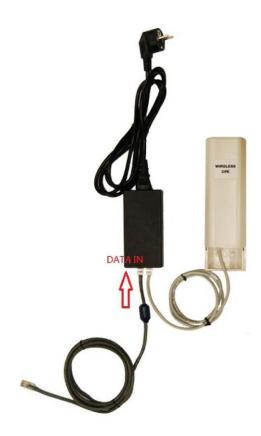
6. Connect the other end of Ethernet cable to a PC or a switch hub. The hardware installation is complete.
