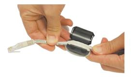
4. Close the core and snap the halves back together.
