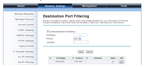
You may create and activate a rule that filters a packet based on the destination port from your local network to Internet. Check "Enable Destination Port Filtering" to activate rule.
