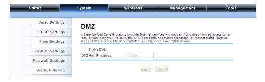
**DMZ Host IP Address:** Enter the local host IP address.
