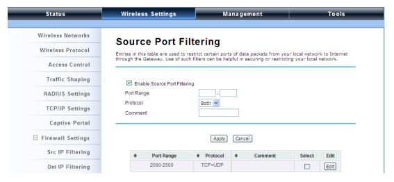
You may create and activate a rule that filters a packet based on the source port from your local network to Internet. Check "Enable Source Port Filtering" to activate rule.
