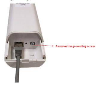
2. Put the grounding wire on the grounding point at the bottom of the ZAC Access Point. Then screw the grounding wire to tighten up.
