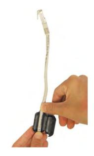
3. Loop the cable around and through the core. This helps "lock" the core in place, and may be required in circumstances with severe interference.
