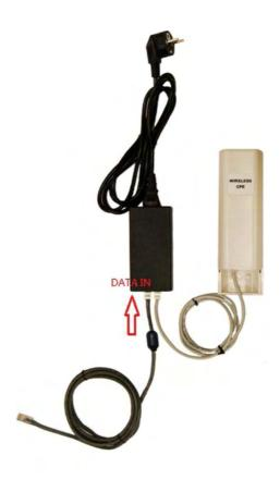
6. Connect the other end of Ethernet cable to a PC or a switch hub. The hardware installation is complete.
