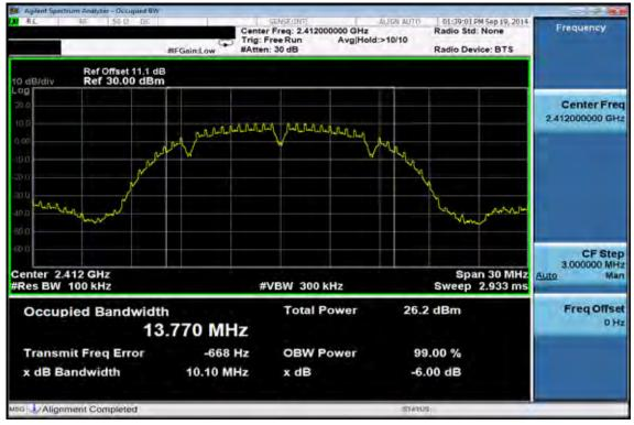
6dB Band Width Test Data CH-Mid
