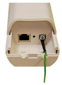
3. Connect the grounding wire to earth ground.
