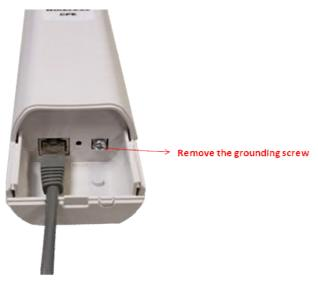
2. Put the grounding wire on the grounding point at the bottom of the ZAC Access Point. Then screw the grounding wire to tighten up.
