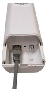
3. Slide the cover back and press down the lock button to seal the bottom of the ZAC Access Point.
