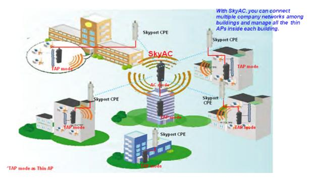
When a thin AP mode joins a wired network, it will start to look for a ZAC Access Point in AC mode. If the thin AP founds the AP controller on the network, it will send the registration request to the AP controller. Once the registration is successfully made, the AP that acts as the AP controller will add the thin AP to its management list and provides it configuration information.
