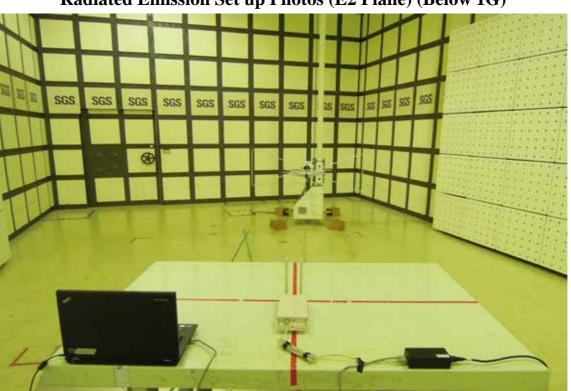
Radiated Emission Set up Photos (E2 Plane) (Below 1G)
