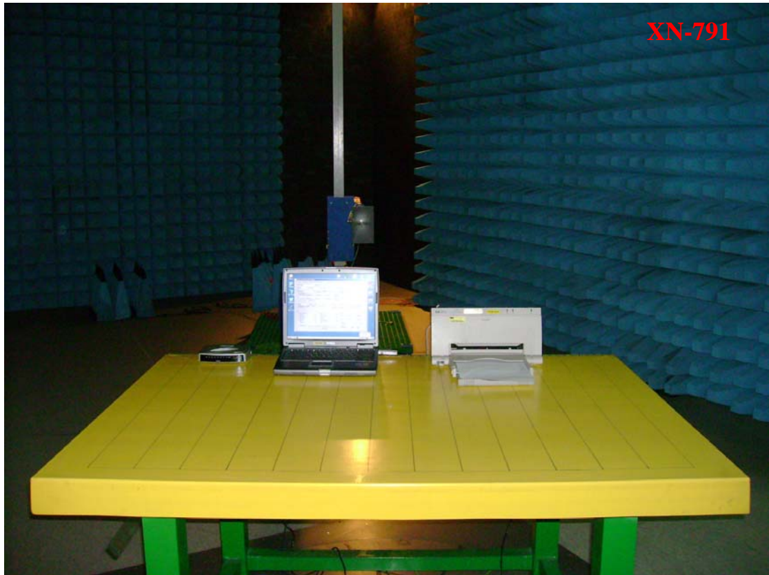
Photo 1: Radiated Emission Test set-up photo
