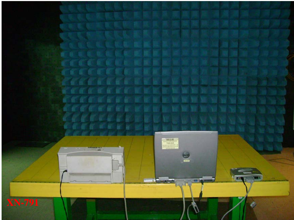
Photo 2: Radiated Emission Test set-up photo
