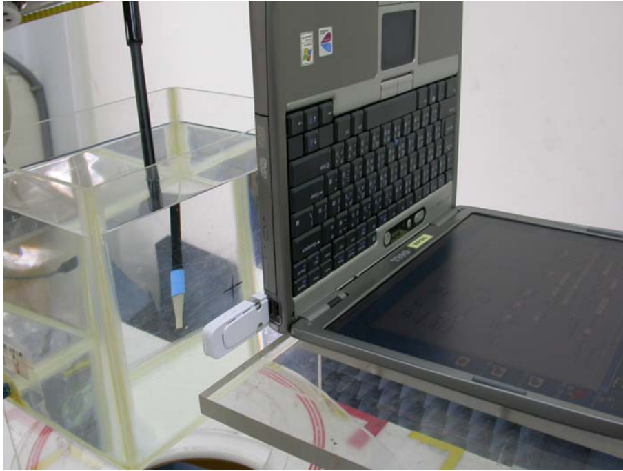
Figure 2: Bottom side of Laptop facing phantom touching
