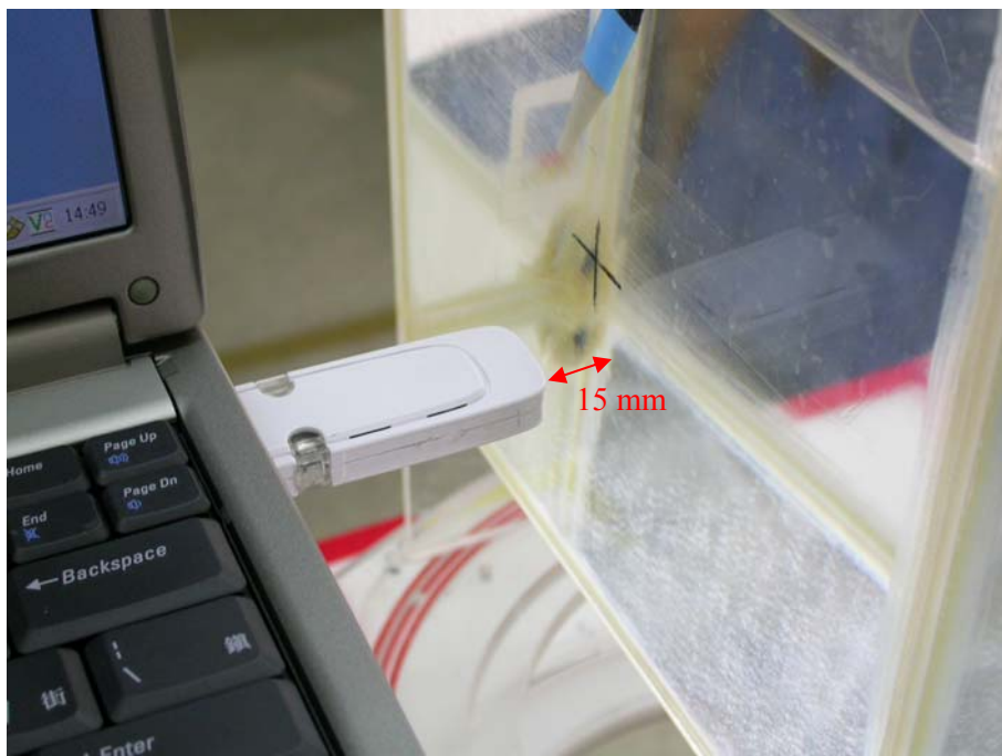
Figure 5: EUT perpendicular to phantom, 15 mm separation
