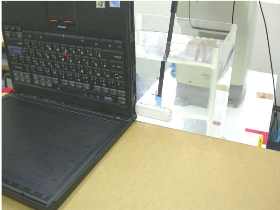
Figure 14: Bottom side of Laptop facing phantom touching
