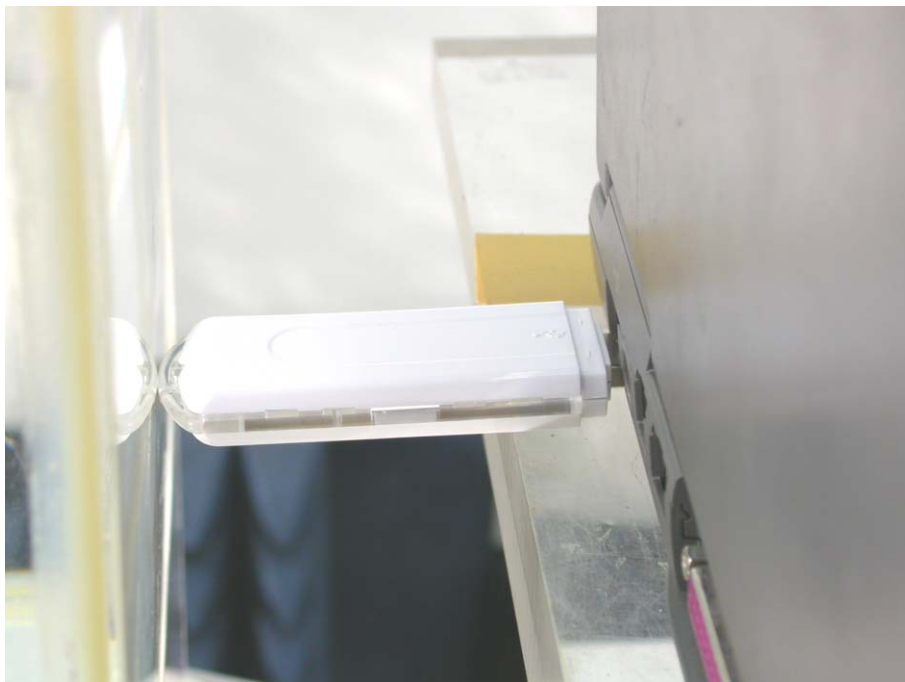
Figure 7: EUT perpendicular to phantom, 0 mm separation-Zoom in
