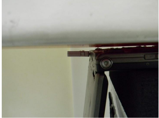
USB Cable Plug-in for USB Configuration 2 (Horizontal Down with Phantom 5 mm Gap)
