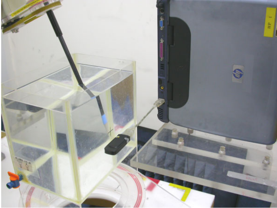
Figure 10: Bottom side of Laptop facing phantom touching (V2)
