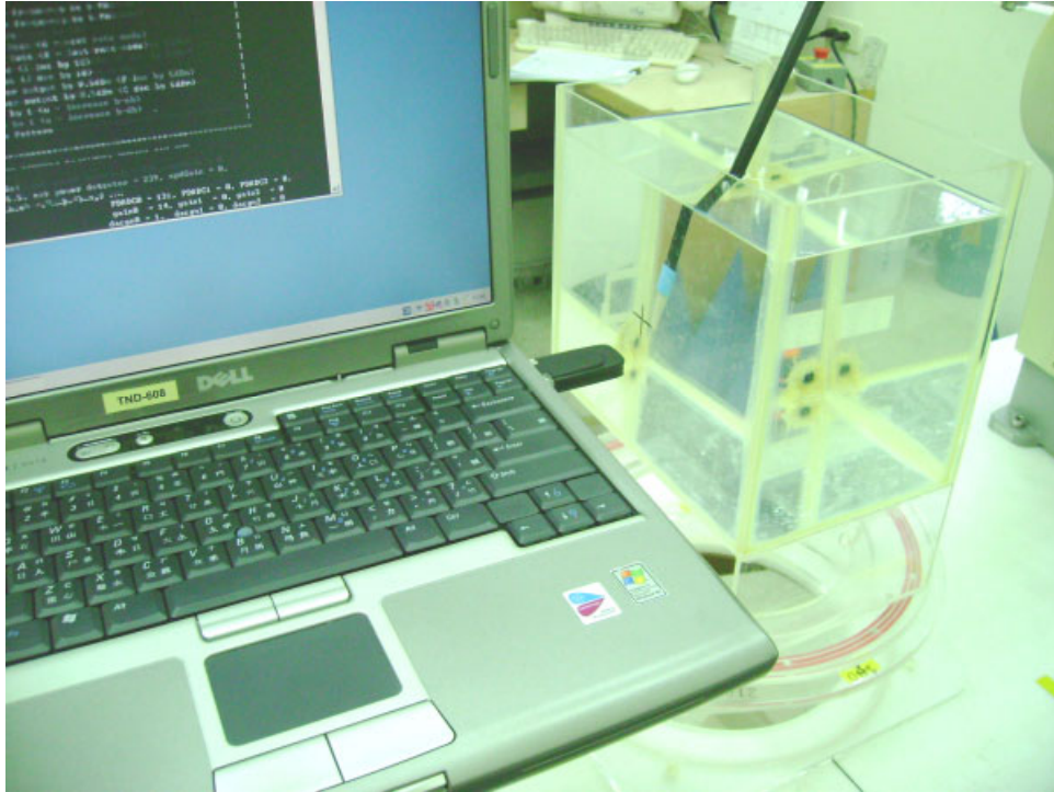
Figure 4: EUT perpendicular to phantom, 15 mm separation
