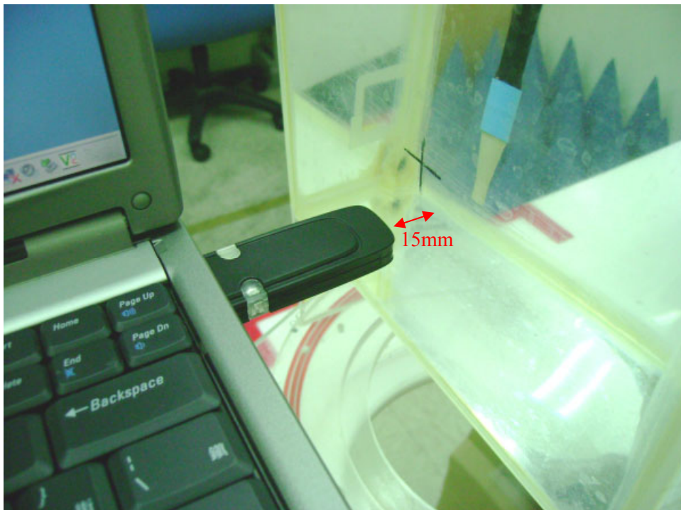
Figure 5: EUT perpendicular to phantom, 15 mm separation-Zoon in
