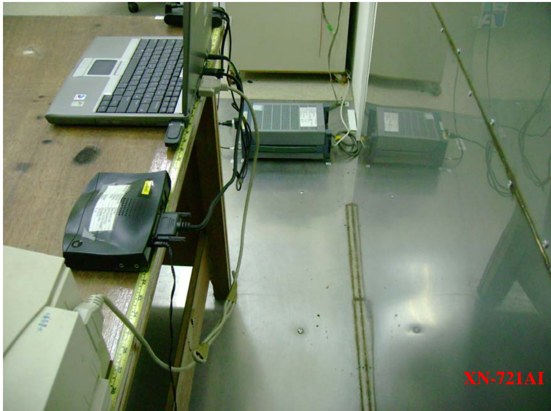
Photo 2: Conducted Emission Test Set-up photo
