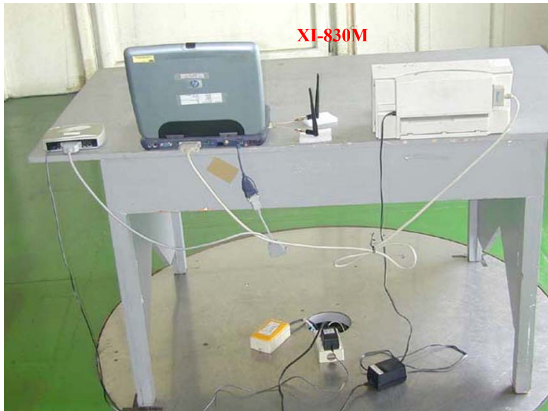
Photo 2: Radiated Emission Test Set-up
