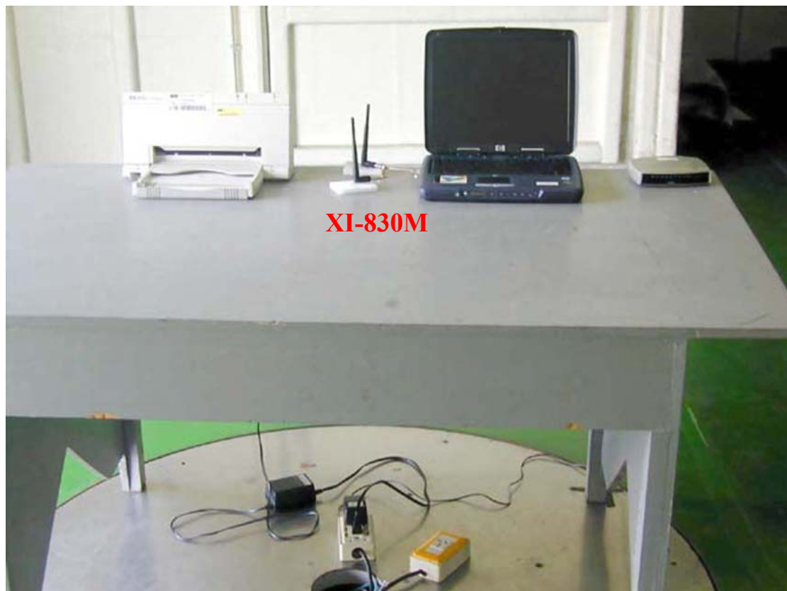
Photo 1: Radiated Emission Test Set-up
