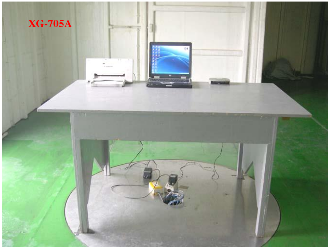
Photo 2: Radiated Emission Test Set-up
