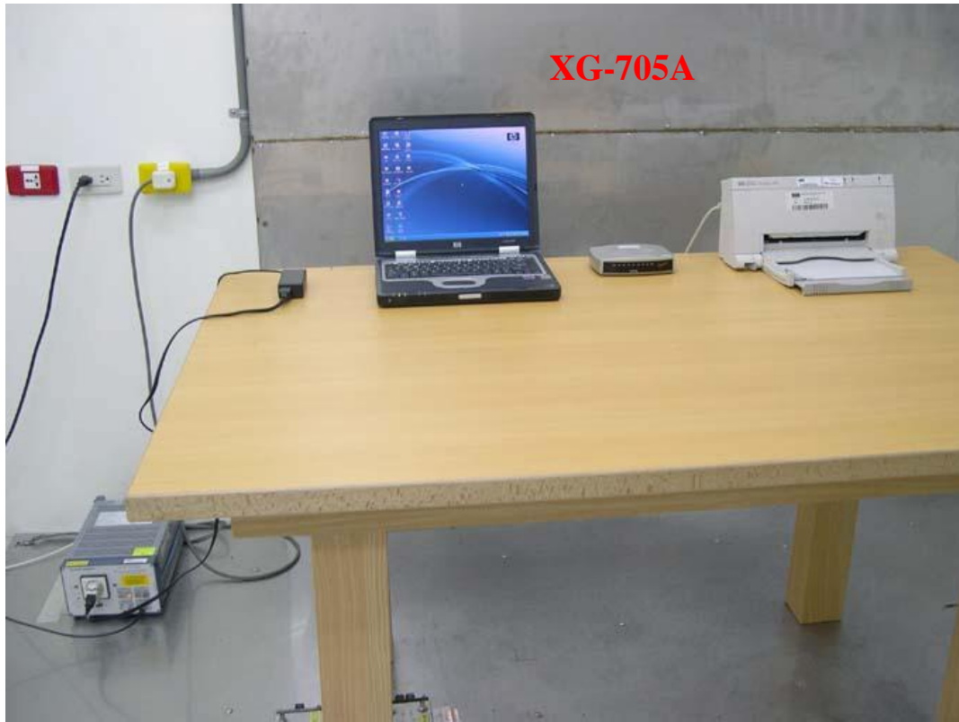
Photo 1: Conducted Emission Test Set-up
