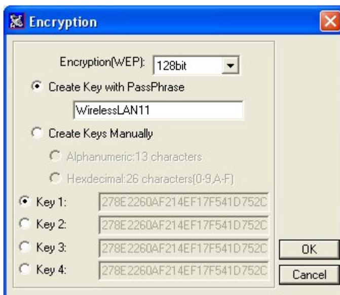
Create Encryption Keys Using a Passphrase (128-bit)
