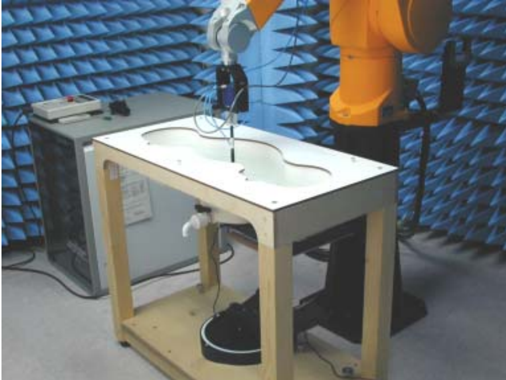
Fig.1 Photograph of the SAR measurement System
