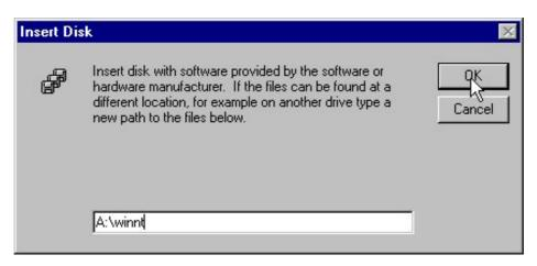
**Step 4:** The Windows will find "**IEEE 802.11 Wireless LAN/CF Card**". Click **OK** and Windows will then copy the necessary files into the system.
