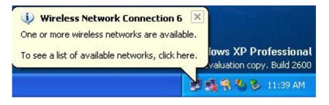
Click on the message and the "*Automatic Wireless Network Configuration* will then appear automatically and allow use to choose to connect a wireless infrastructure network (Access Point), shown as the below figure. You may click the **Advanced** button to make advanced configuration for the Wireless LAN CF Card, shown as below.
