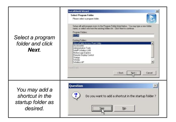
Upon completion, go to **Program Files** and run the WLAN Utility and its icon will appear in the **System Tray** in the bottom right corner of your task bar. Clicking on the icon will open the configuration window. When you minimize the window, the system tray icon will be loaded in the System Tray again.
