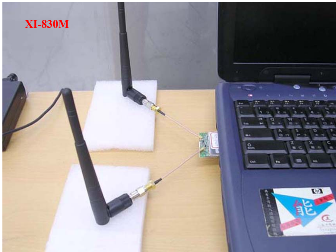
Photo 3: Conducted Emission Test Set-up
