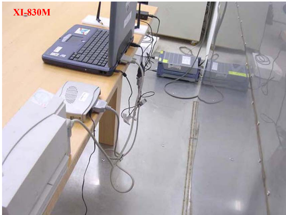
Photo 2: Conducted Emission Test Set-up
