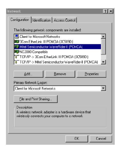
➤ Click on the "Remove" button. If you have hardware profiles installed, you will be asked if you want to remove all occurrences of the adapter, as shown below. Click on the "OK" button to uninstall the driver.
