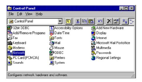
From the Network control panel, select the Mitel Semiconductor WaveRider-II adapter. Be careful to select the correct adapter and make sure that the picture of an adapter is next to the description of the adapter, as shown below:
