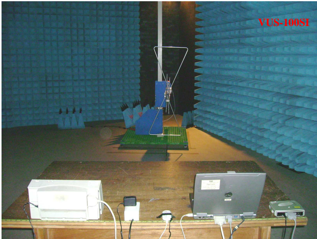
Photo 2: Radiated Emission Test set-up photo
