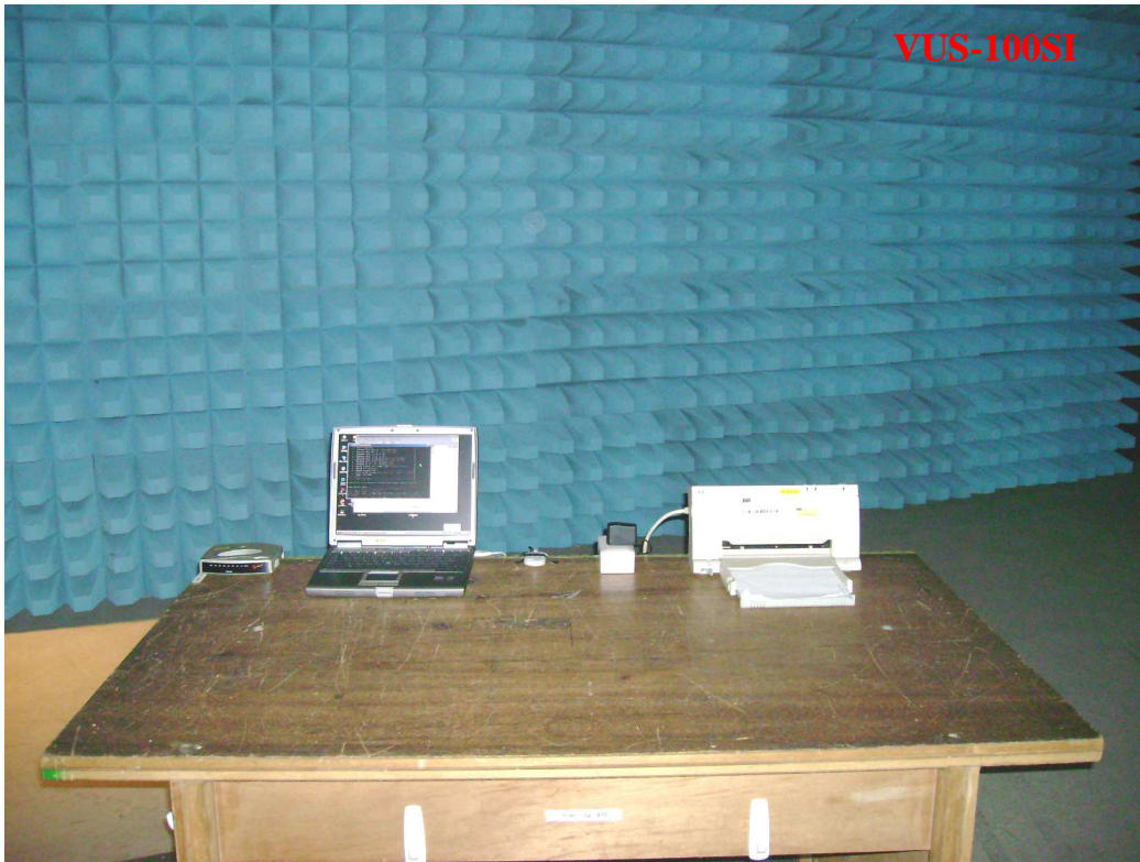
Photo 1: Radiated Emission Test set-up photo
