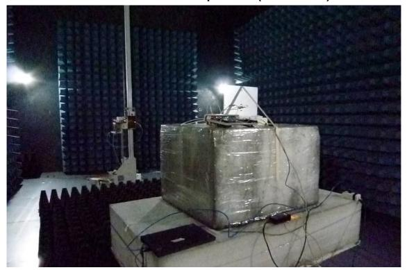
Radiated Emission Set up Photos (Front View)
