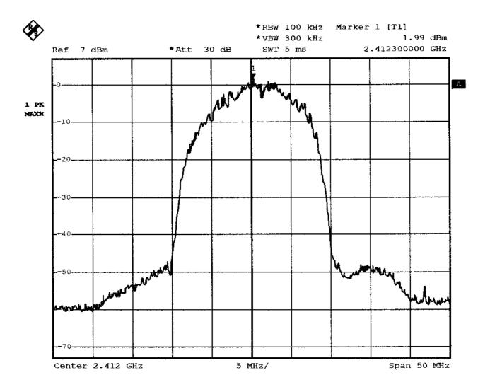
Comment A: RF conducted spurious at low channel external att.=3dB cable loss=2dB
